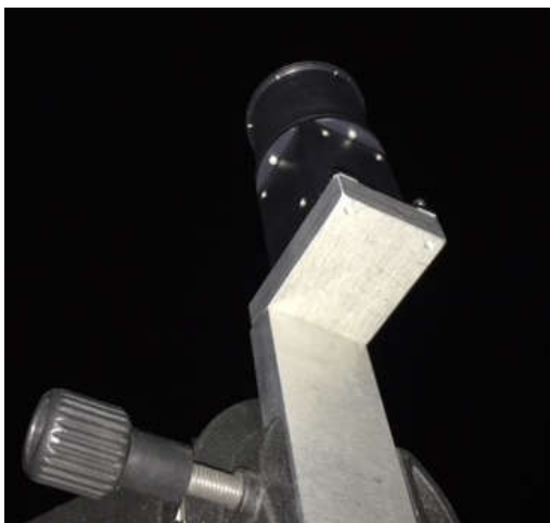
Fig. 6 - Nano star tracker AZDK-1 on a tripod during the field tests and the resulting image of the Pleiades cluster with an exposure time of 0.1 seconds
